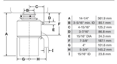
NOTE: Plumb 1-1/2" (38.1 mm) waste line to prevent standing water in disposer motor housing.
