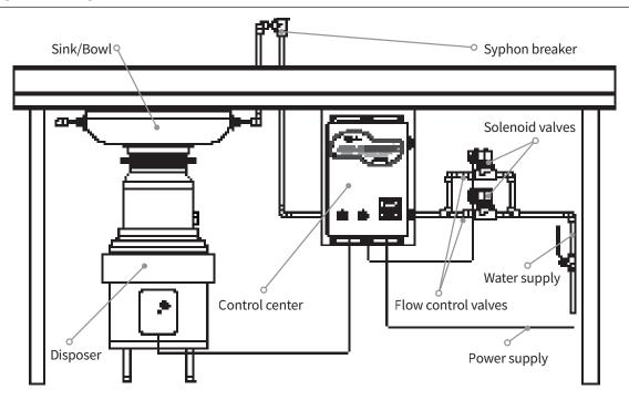
Aquasaver is to be installed 38.1mm back from the edge of the workstation bench to protect from water overflows.
