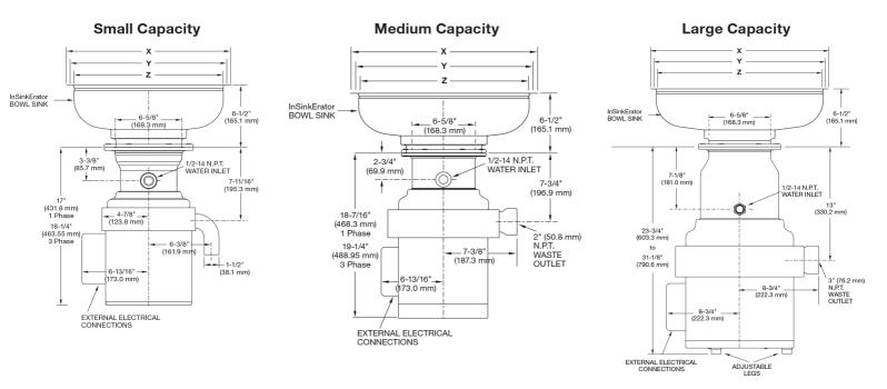
If mounting directly to a sink, use dimension chart below for adaptor height in place of InSinkErator bowl sink height. *IMPORTANT:* #5 adaptors and #12 bowl only available with SS-100.
