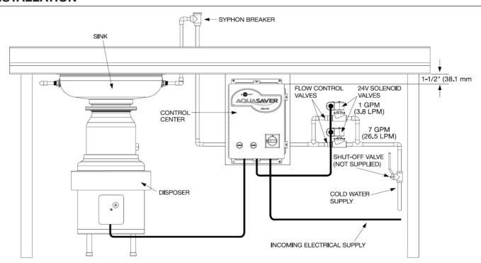
Aquasaver is to be installed 38.1mm back from the edge of the workstation bench to protect from water overflows.
