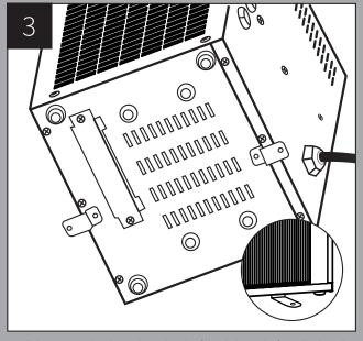
Install the mounting bracket to the underside of the chiller on the fan grill side and opposite side.
