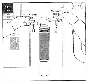
\* NOTICE: Property Damage. Top surface of cartridge will be flush with bottom of filter head when fully engaged.
