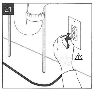
\* NOTICE: Property Damage. Do not use an extension lead with the tap. (A standard earthed outlet within 760 mm (30") of the tap is required under the sink.)
