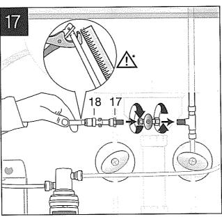
NOTICE: Property Damage. Tube runs need to form to the cabinet's contours to allow storage space with no sharp bends. Tubes need clean, perpendicular, burrfree cuts to ensure a true fit. Join remaining tube to cold water supply only.
