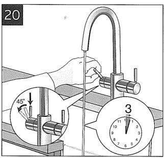
**Note:** Water will be cold at first, Allow 12-15 minutes for water to reach target temperature. Gurgling or hissing is normal during the initial heating cycle.
