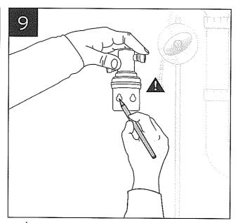
**WARNING.** (Personal Injury) Do not locate filter above an outlet or other electrical device. Install head and bracket so that connections require no stretching, kinking or pinching of tubing.
