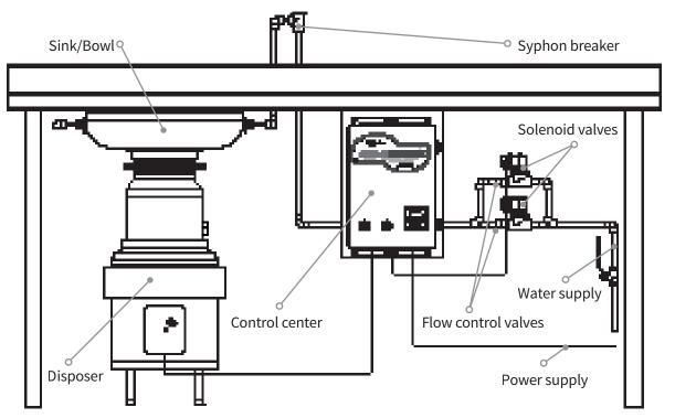
Aquasaver is to be installed 38mm back from the edge of the workstation bench to protect from water overflows.
