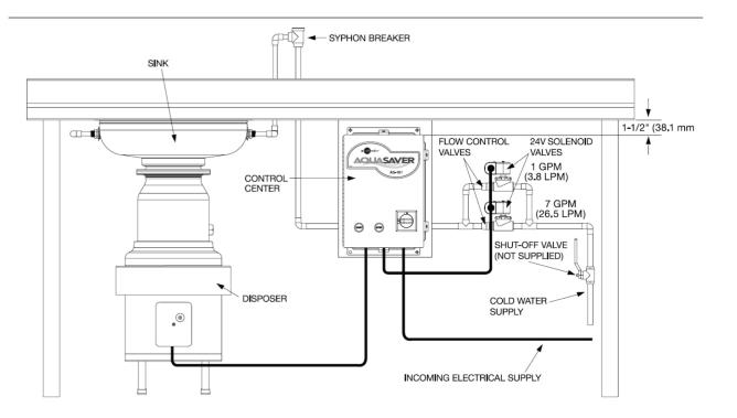
Aquasaver is to be installed 38mm back from the edge of the workstation bench to protect from water overflows.
